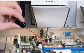
The **Closed-Loop, Non-Contact IR Pyrometer** monitors and controls the ramp-rate and temperature of the component in real time, by controlling the top and bottom heaters' output throughout the reflow process.
